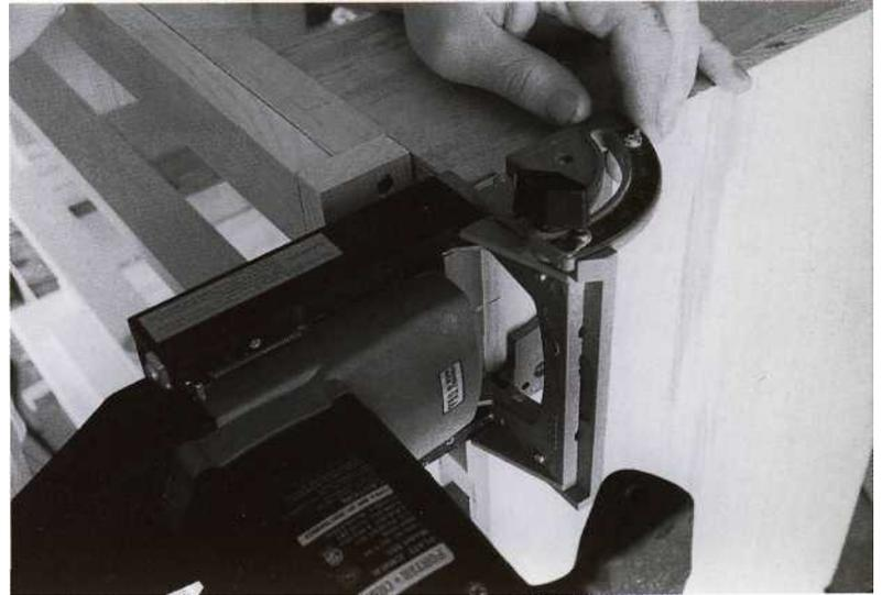
Cut the biscuit slots to the pilasters and side panels
