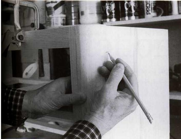
Once the spacers are securely fastened to the carcass, set the pilasters in place and mark them, one side only, and the carcass for biscuit slots.
