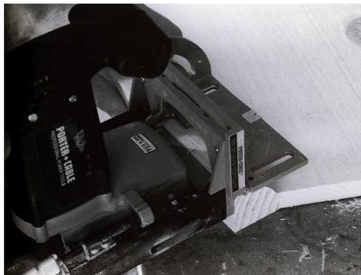
Take extra care to ensure the plate jointer is square to the work when milling the biscuit slots to the pilasters.
