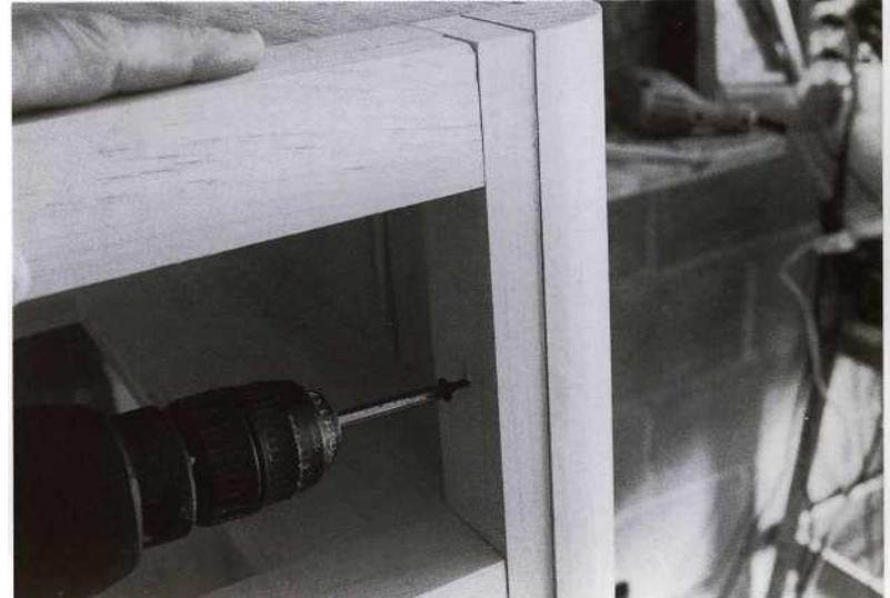
Glue the pilasters in place to the sides of the carcass and, from the inside, using glue and no. 6 screws, secure the pilasters to the spacers already screwed in place.
